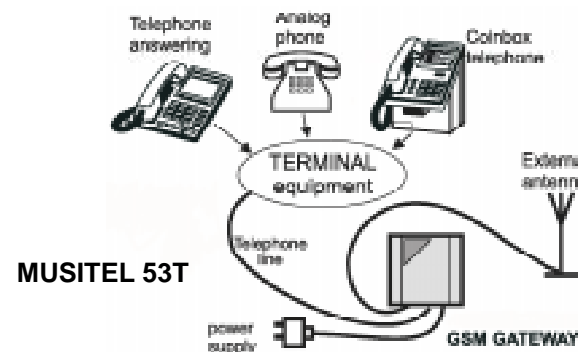
Fig. 3.: Optional Connection of More Terminal Equipment
