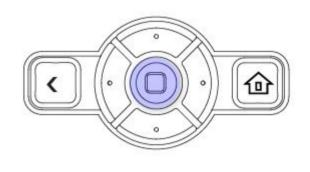
Use the left and right soft key below the screen to select a new status and confirm using the select key (in the middle of the navigation keys)
